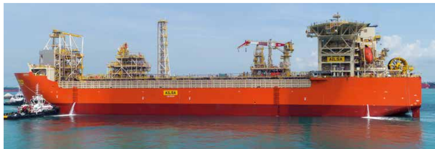
Delivered to MODEC, the newbuild FPSO Ailisa is the world's first with a 40-year hull lifespan
