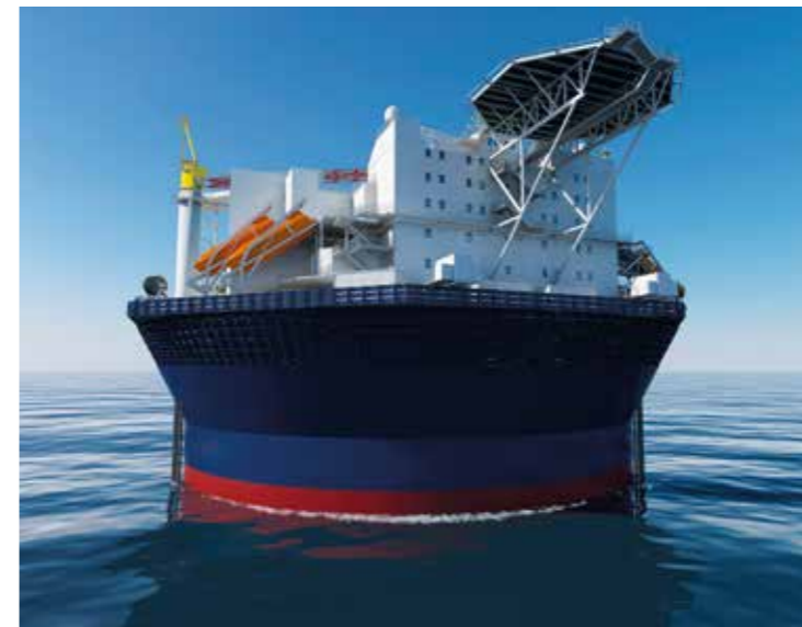
Sevan SSP: Innovative circular hull as a cost-effective alternative to traditional ship-shaped, turret moored designs
