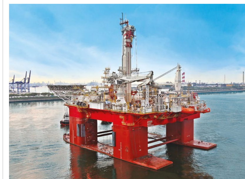
Q7000 well-intervention semi-submersible rig delivered to Helix Energy Solutions
